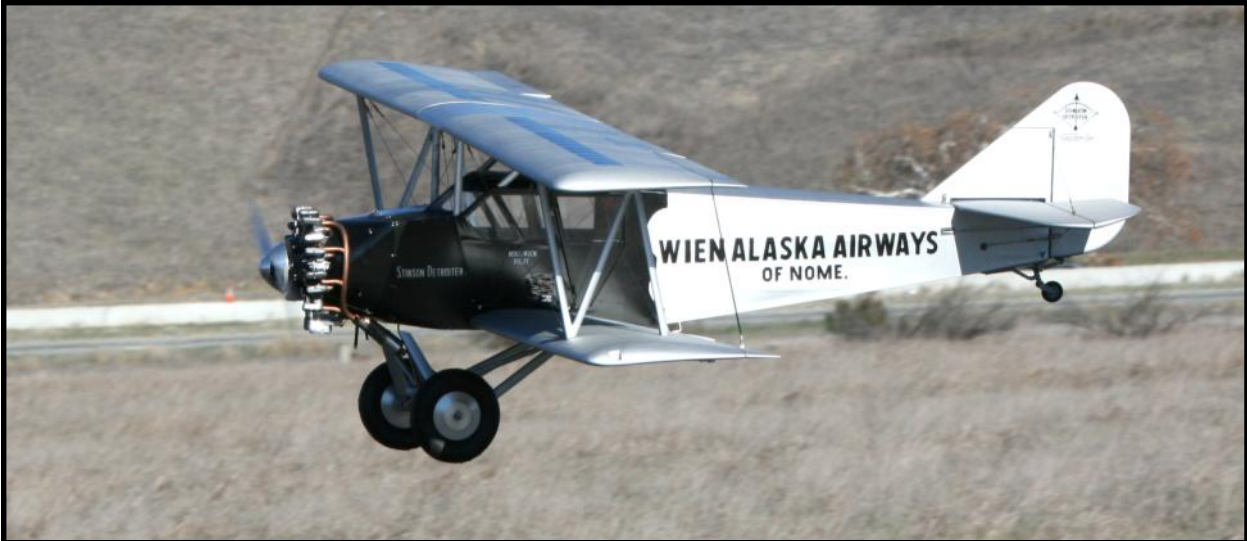
Bob Zuk's SB-1 Stinson Detroider, circa 1920s. It was the first biplane in the U.S. with an enclosed cabin which allowed it to be a commercial plane in Alaska. It's 1/5 scale, wingspan 86 in., wt. 20 lbs. with a Saito 220. The kit was manufactured by 3 Saebees. Would you believe it is an ARF? PR photo.
